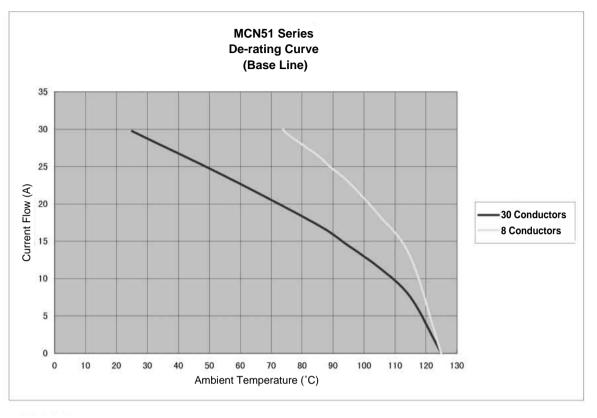
Measurements were made with 12 AWG wire connected in series to all contacts.
