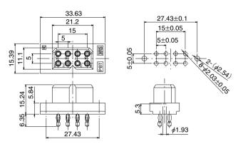
Copper plating thickness :  $70 \pm 10 \mu m$ Solder plating thickness : 5 to 10  $\mu$ m Board thickness : 3.2 mm min.
