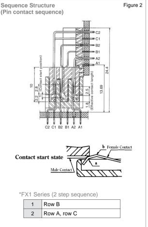
Setting row B to ground, if active cable insertion and extraction are performed as power supply, arc will occur between contact and contact. The row B contact structure is constructed to separate arc occurrence point a and normal contact point b, and minimizes affects on the contact.
