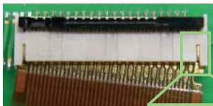
Incomplete FPC insertion
