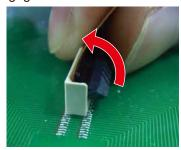
During the design phase of the PCB layout, make sure to incorporate enough space to engage/ disengage the actuator on this connector when inserting or removing the FPC.
