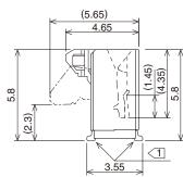
Note 1>: The coplanarity of each terminal lead within specified dimension is 0.1mm Max.
