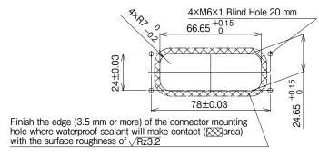
Remarks: The dimensions of the panel mounting hole are the dimensions when seen from the plug mating side.
