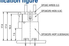
Note: The retainer can be used on both the standard and R type housings.
