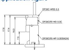
Note: The retainer can be used on both the standard and R type housings.
